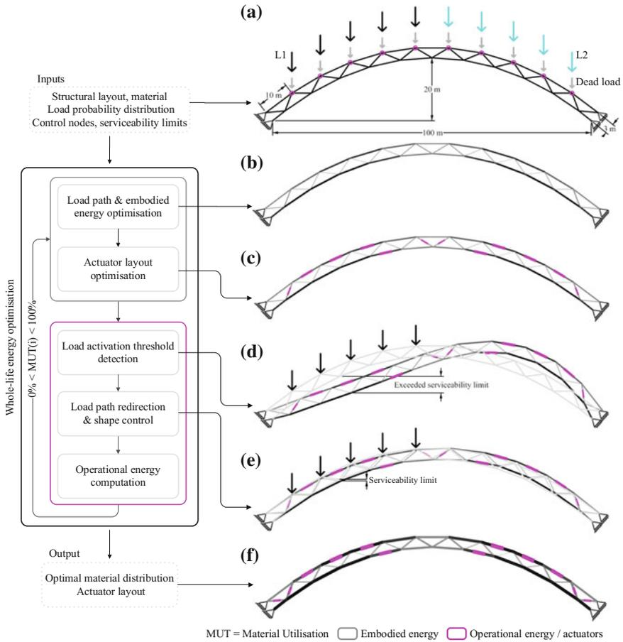
**Fig. 8.2** a Initial layout and controlled nodes; b minimum embodied energy design  $MUT = 100\%$ ; c optimal actuation layout  $MUT = 100\%$ ; d deformed shape; e controlled shape; f minimum whole-life energy design  $MUT < 100\%$
